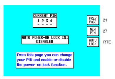
Screen 26: PIN Change & Power-On Lock Enable Screen
