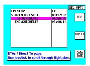
On entry to the adjacent screen the cursor highlights the waypoint in MAGENTA that is currently being navigated to. If ATC clear you to END: CHICHESTER, for example, you can use the Direct-To waypoint function to amend the routing quickly without having to edit the Flight Plan. Use the joystick to move a BLACK highlight over END: CHICHESTER, then press **DIRECT TO**. This function is not available in External GPS Mode.
