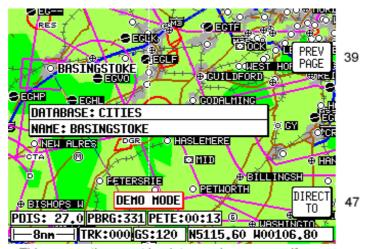
This screen times-out back to previous screen if joystick is not moved or key is not hit for 30 seconds Screen 40C: Map Mode General Information Screen
