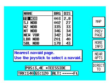
The desired information will be presented dynamically as a bearing and distance from your present position. Any displayed item can be instantly navigated to by pressing the **DIRECT TO** key. Alternatively the **MAP** key can be used to return the user to MAP mode.
