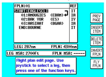
and press **DELETE ITEM**. A flight plan can be systematically built using the **INSERT ITEM** key.
