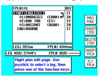
Ensure that the leg arrow is pointing at the initial leg that is to be flown and press **FLY FPLN**. The unit will immediately revert to map mode with the navigation information showing, using the preselected MAP mode presentation
