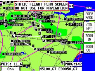
To systematically create additional legs, draw a line from the waypoint marked (E), with the pointer, to the next waypoint and press **ADD WPT** again. You will notice that the last point in the flight plan will always be labelled (E). Once you have finished building the flight plan press **PREV PAGE**, to detach the pointer from the flight plan. This key, if pressed again will return to the screen entered from, saving any changes made.
