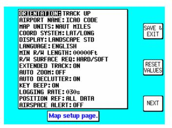
The initial screen is reached by pressing **SET UP** in MAIN MENU, followed by **MAP SETUP**. The subsequent screens are reached by pressing the **NEXT** key.
