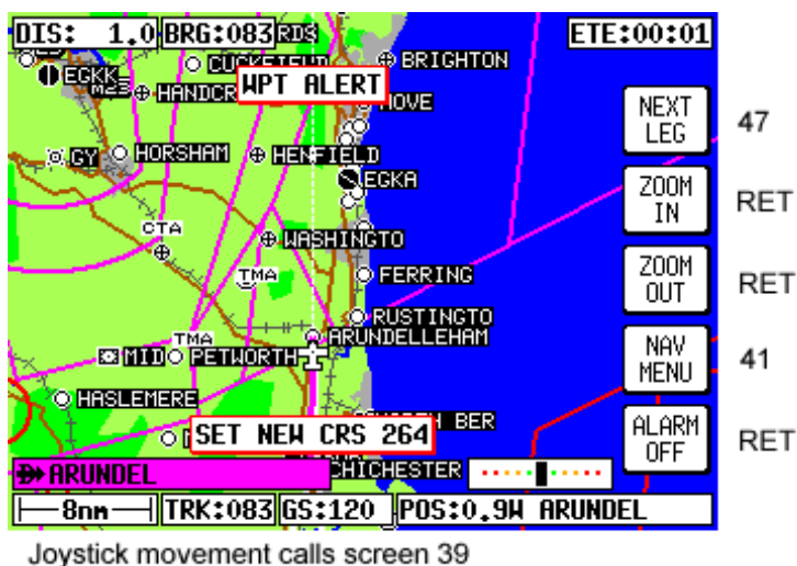
Joystick movement calls screen 39 Screen 48: NAV Information and WPT ALERT Flags Showing – En-route Screen
