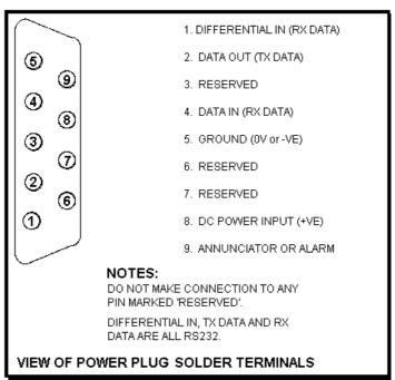
The data presented across the data output pins is controlled by the settings on Screen 35, Data Input/Output Setup and Test Screen. If you want to connect an external audio annunciator to your unit, do so in accordance with the following drawing and activate it's operation on Screen 23, NAV Mode Customisation Screen by setting EXTERNAL ALARM to ON.
