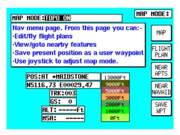
In all three modes there are a further two options which are either TOPO ON or TOPO OFF. In the TOPO ON mode all classes of data can be set to a specific colour. In the TOPO OFF mode all cartographic data is automatically removed and the Jeppesen NAV Data is presented on a black background.
