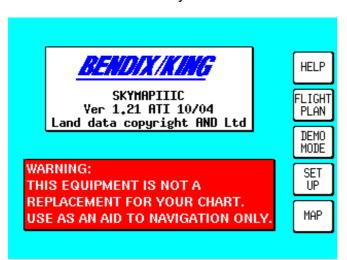
The appropriate key labels for a particular page are configured in software and drawn alongside the appropriate black key. The rotary ON/OFF switch is used for adjusting the brightness of your screen.
