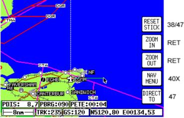
This screen times-out back to previous screen if joystick not moved or a key is not hit for 30 seconds
