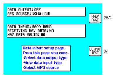
Screen 35: Data Input/Output Setup and Test Screen
