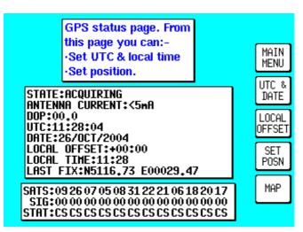
Altering UTC & DATE: Select UTC & DATE, followed by ADJUST UTC. Use the joystick to adjust the time, and then press SET. Now select ADJUST DATE and use the joystick to adjust the date, and then press SET followed by GPS STATUS. Option not available after the GPS has determined the correct time.
