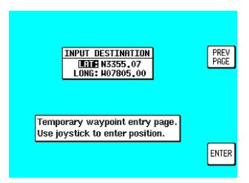
Then press TEMP WPT and use the joystick to dial in the required latitude and longitude, followed by ENTER. The unit will then provide you with full navigation information to reach this point.
