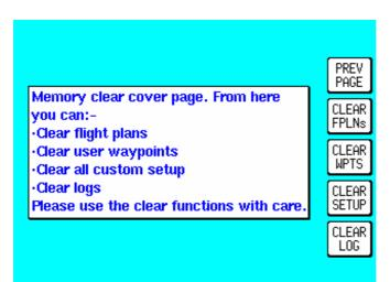
Each block of memory in your unit can be cleared down individually. CLEAR FPLNs will remove all your flight plans. CLEAR WPTS will remove all your user waypoints. CLEAR SETUP will restore all the default settings in MAP SETUP and NAV SETUP. CLEAR LOG will clear the last flight information, the 2000 logged flight data points and all running timers.
