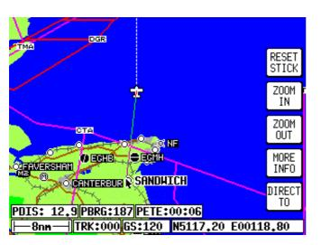
In MAP mode use the joystick to move the pointer to the desired location, or obtain the latitude/longitude and bearing/distance from present position.
