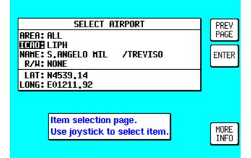
whether it is to find out airport frequency information, or select a DIRECT TO point or when creating a flight plan. In each case the adjacent screen will appear. Use the joystick to highlight the database in which the desired item is contained and press **SELECT.**
