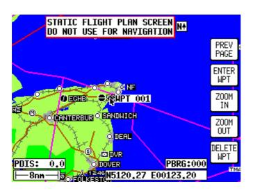
A user waypoint can then be created as a distance and bearing from the displayed position or as a latitude/longitude. Press **ENTER WPT** to save the user waypoint to the first available memory location. An unwanted user waypoint can be removed by moving the pointer over it and pressing the **DELETE WPT** key.
